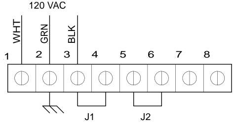
All circuits should be fused or protected by a circuit breaker (10Amp maximum)
